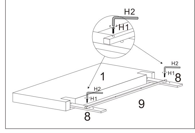
Step5 Please connect the corresponding headboard support (8) to the corresponding bed side board (13/14). The headboard support (8D) connects the bed side board (13) and the bed side board (12). The headboard support (8A) connects the bed side board. (14) with the bed side panel (5), and then tighten the corresponding screws with (H2)
