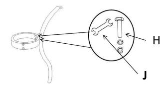
Loosely attach the Central Round Support Ring(C) to Table Legs(B) using washers, Spring Washers, and Hex Bolts(H), with the Spanner(J).
