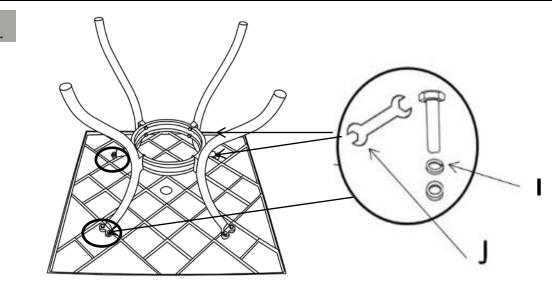
Lay the Table Top(A), top facedown, onto a flat, soft, clean surface. Attach the Table Legs(B) to the the Table Top(A) using Washers, Spring Washers, and Nuts(I) with the Spanner(J).
