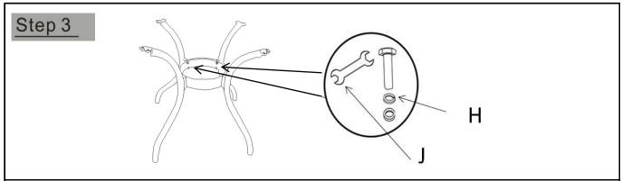
Repeat step 2, attaching the remaining 3 legs to the Central Round Support Ring(C)
