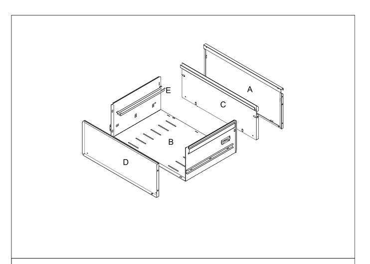
Step1:Install Drawer Face Panel (A) and Drawer Body (B) and ensure that five clips on the panel to insert the Drawer Body (B) and fold the snap joint.
