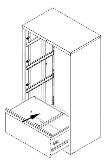
Must step: A First slide the steel ball to the front of the cabinet's outer slide.
