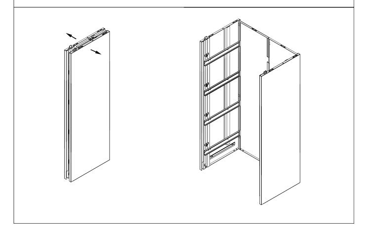
Step2: Install the Base Board (K); first of all,hold up the Base Board (K) and the clip shall form a right angle. Ensure that it can be clipped into the card slot on the back and two sides of the Base Boards (K) can be clipped into the side plates.
