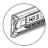
B: Insert the inside railway course on both sides of drawer on the outside railway course of cabinet at the same time. Two people must put the drawer flat and insert it slowly and synchronously. After inserting it to the end, pull it out slowly twice, the slide track works normally. If it works fails, please follow the slide track removal instructions, open it and reinstall it.
