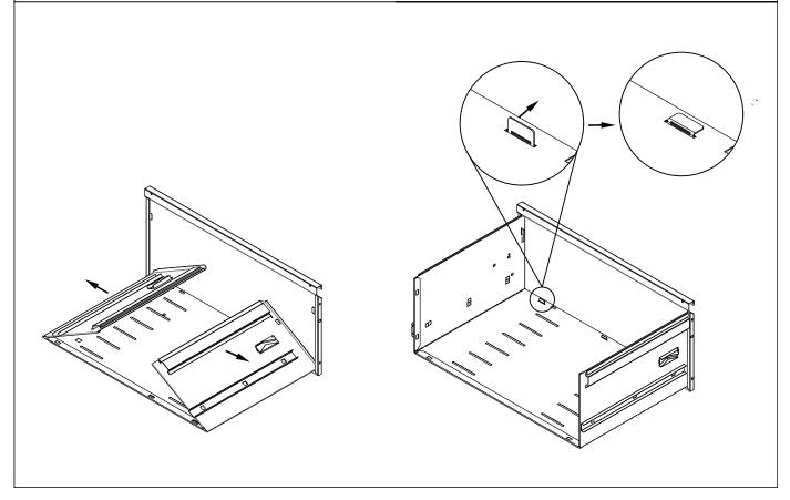
Step2:Install Front Guard Panel(C) and use the screwdriver to jack up four limitswitch buckles on Front Guard Panel(C)
