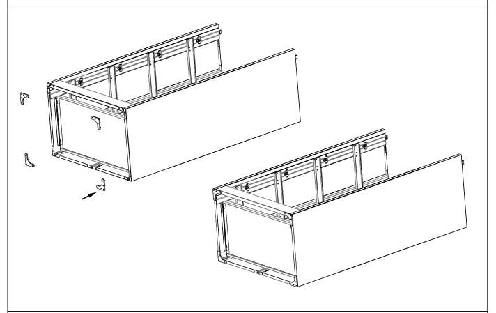
Step 5: Install Top Board (J); fold straight clips on the left side (F), the right side (G), the left back (H) and the right back (I). After it is clipped to the Top Board slot, flatten the clip. Ensure that the spring shaft of the Top Board linkage rod can be clipped into locking rods on the left side and the right side.
