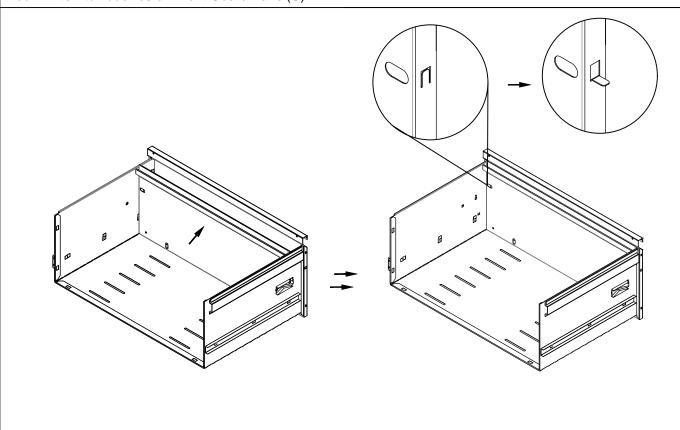
Step3:Install the Rear Guard Pabel(D)and ensure that the Rear Guard Pabel(D)is clipped into the Drawer Body  $\,$  (B)  $\,$ .
