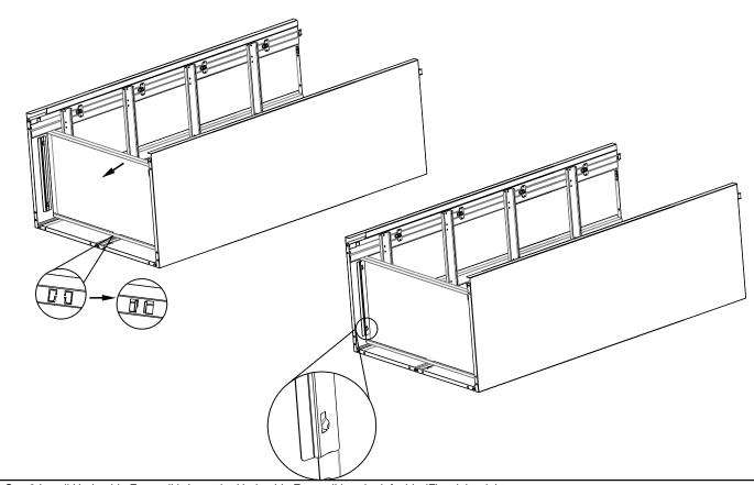
Step3:Install Underside Frame (L) .Insertthe Underside Frame (L) to the left side (F)and the right side (G) and push clips on the left and right side frames into the Underside Frame.
