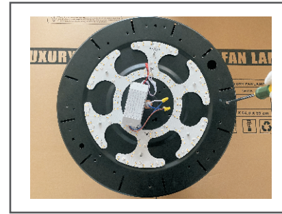
Step 4. Remove the main engine chassis screws.
