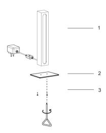
Install the Light Frame (1) to the base (2) until tight through screws (3).
