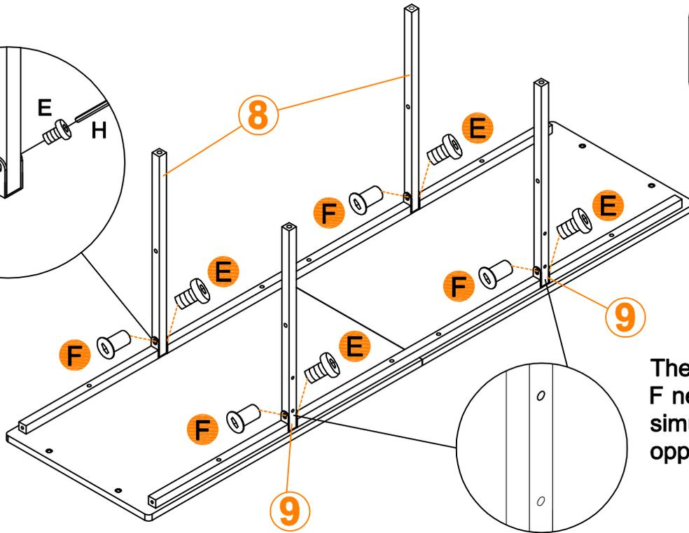
The screws E and bolt F need to be tightened simultaneously in the opposite direction.
