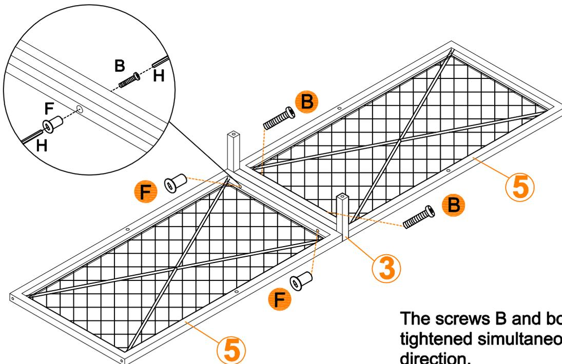
The screws B and bolt F need to be tightened simultaneously in the opposite direction.
