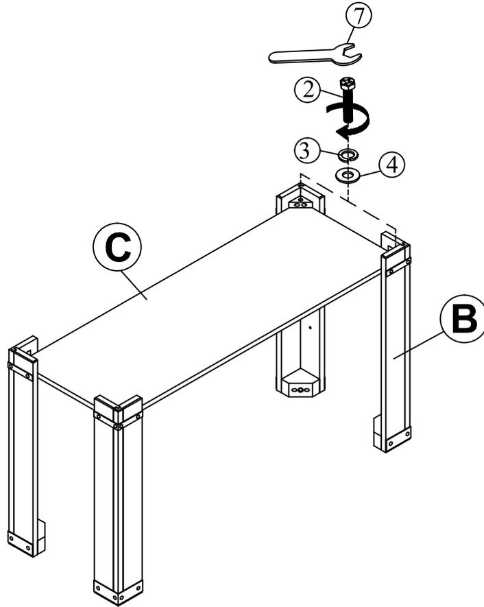
**STEP 2 :** Place the Table Top (A) on the floor with a piece of cloth or carpet underneath to prevent finish from scratching. Attach the assembled base in Step 1 to the Top by using Flat Washer (4) Lock Washer (3) and Long Bolt (1) through the corner block. Secure well by Wrench (7).
