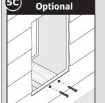
**5C Optional:** Use the 2 drywall screws (supplied) or 2 wood screws (optional) to fasten the outer portion of the support.
