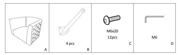
Note: Put all the screws into the hole site, And then tighten them. Do not tighten one by one
