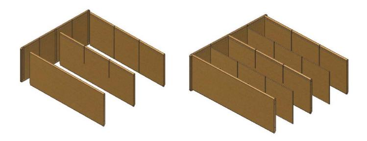
**Step 1:** Attach **Top, Bottom,** and **5/8**" **thick shelf** into a **Side** piece using **(6)** supplied **Hex screws** and **Allen wrench** provided. Back grooves in Top and Bottom, -cuts that go all the way through from short end to short end, align with 3/8" deep back groove in Side piece. Back grooves face inwards torwards middle of Side piece. Slots in 5/8" thick shelves also point torwards 3/8" deep back groove in Side piece.
