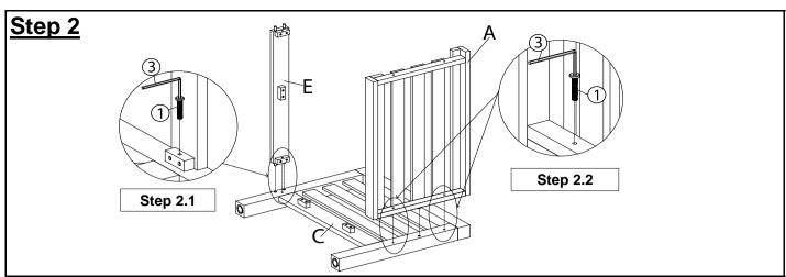
Place the Left Arm Panel (C) with inside face skywards onto a clean, soft surface to avoid any scratches or damages to the product.
