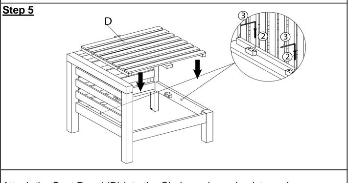
Attach the Seat Panel (D) into the Chair as shown in picture above. Affix Seat Panel (D) with Chair by using Screws ((2)) and Allen Key ((3)). Note: Using Screws ((2)) from inside to outside of Seat Panel (D) **DO NOT FULLY TIGHTHEN SCREWS.**
