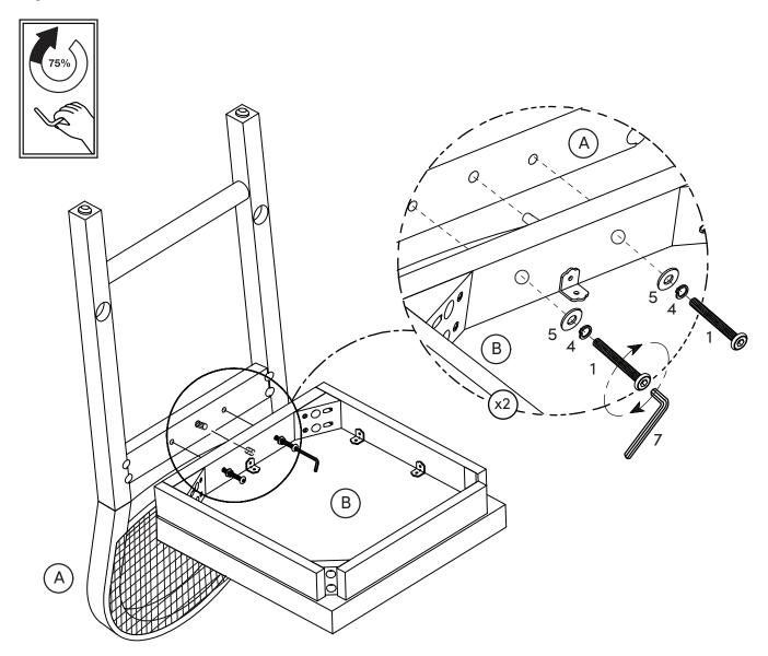
Match the sticker on the bottom of the Chair Back Assembly (A) with the sticker on the corner block of the Seat Cushion Assembly (B).
