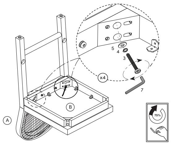
Do not overtighten hardware. Tighten to 75% for now.
