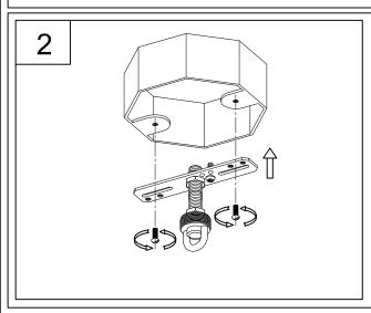
2. Attach assembled parts from step 1 onto junction box, using the mounting screws supplied with the junction box (not included).
