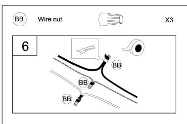
3. Strip 3/8" of insulation from the electrical wire ends. Using wire nuts (BB), connect RIBBED fixture wire to the WHITE supply wire from the junction box; connect the SMOOTH fixture wire to the BLACK supply wire.
