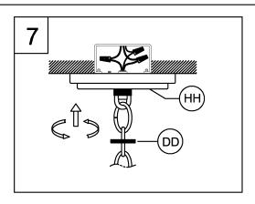
7. Tuck the wires into the junction box and slip the canopy over the chain holder. Thread the screw collar (DD) onto the chain holder to secure the canopy tightly to the ceiling.
