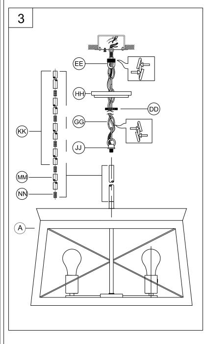
4. Assemble nipples (KK) and pipes (HH, JJ) together to achieve a desirable hanging length. NOTE: Also at this time, you may choose to shorten the chain length and electrical/ground wires, but be sure to leave 6" minimum wire lengths beyond the canopy for connection. When completed, pass the wires through the assembled pipe lengths.
