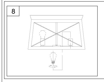
8. Screw lamps (not included) into fixture socket. Use 100-watt MAX incandescent medium base, SBCFL or SBLED.
