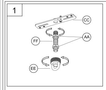
1. Screw threaded nipple (FF) into mounting plate (CC) several turns. Use one hex nut (AA) to secure parts tightly. Screw one hex nut (AA) and chain holder (EE) onto threaded nipple (FF). Tighten the hex nut against the top of the chain holder.
