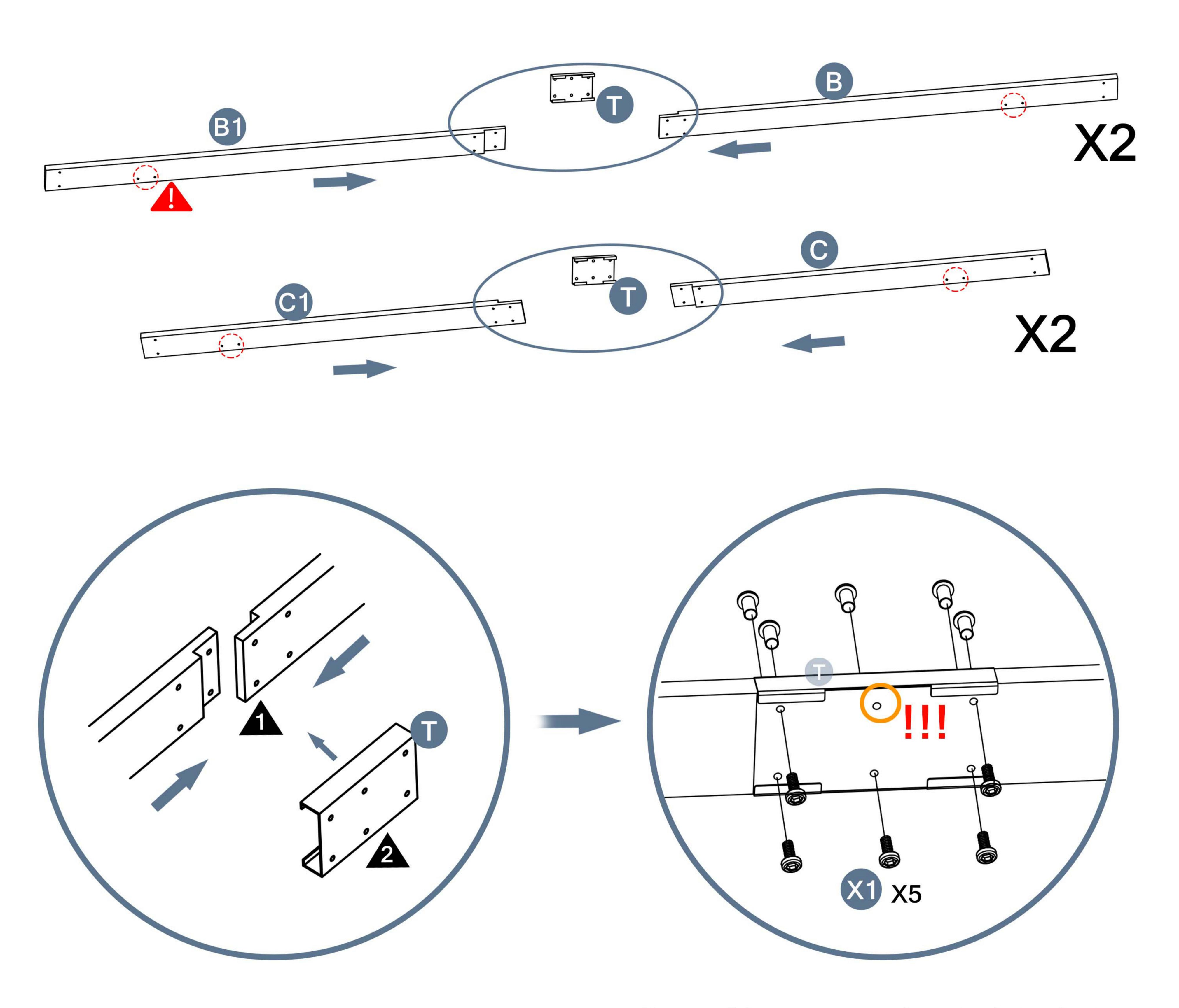
Be careful not to screw into the holes in the yellow circle at this step and screw at step 5.
