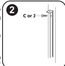
Install second screw (**C**) in top of hinge bracket securing it to the wall.
