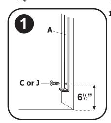
1. Install hinge bracket (A) to wall (stationary side of gate) using Phillips screw (C) drill pilot hole 6½" above floor surface. (Use ruler on left edge of this sheet to measure from floor).
