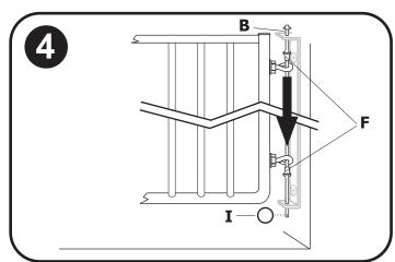
4. Hang gate by inserting hinge rod (**B**), through top of mounted hinge bracket (**A**), through upper plastic shoulder washer (**F**), through both eye bolts, through lower plastic shoulder washer (**F**), and finally through bottom of hinge bracket. To secure hinge, insert key ring (**I**) through hole in end of hinge rod. Gate can be mounted at angles up to 30 degrees.
