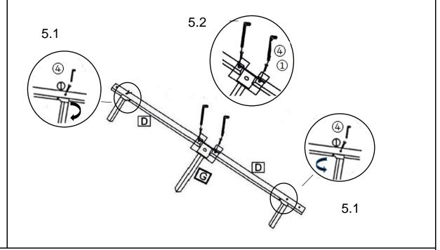
**5.1)** Align Vertical Slats with Legs(D) and pull legs along the direction of the arrows slowly as shown.
