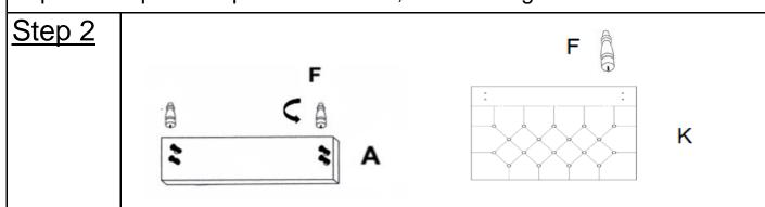
Place the Footboard(A) with the bases facing skywards. Install the Legs(F) at the bottom of the Footboard(A) by inserting the threaded stem into the threaded mounting postion on the Footboard(A). Tighten by turning the Legs clockwise.
