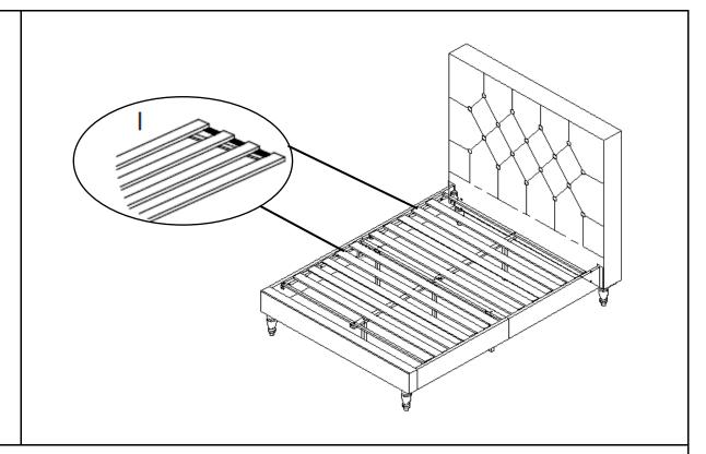
Now tighten all Bolts fully at all joints in a sequential manner. Then, place Wooden Slats(I) onto Bed frame to make sure Wooden Slats(I) fix well.
