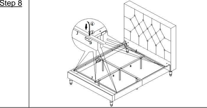
Attach Cross Slats(J) to Vertical Slats with Legs(D) and Side Panels(B) and Side Panels(C) using Bolts(1) with Allen Key(4).
