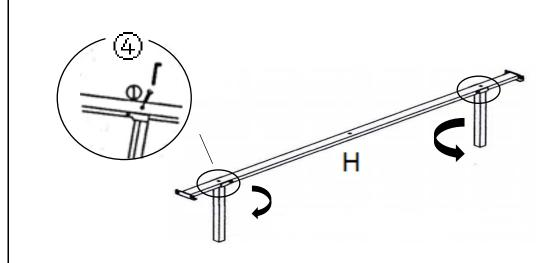
Align Middle Support Slat with Legs(H) and pull legs along the direction of the arrows slowly as shown.
