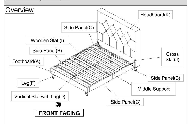
This Bed has multiple parts and may require up to 30 minutes to assemble. To give you an overview of the Bed parts, the above picture is to help you put the various Bed parts into perspective.
