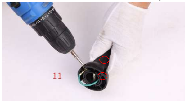
13. Remove 2 screws on the hanger ball
