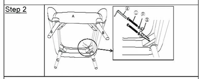
Insert the Back Leg(C) into the mounting position of Chair(A), and attach using Bolts(①), Spring Washers(②) and Washers(③) with Allen Key(④).
