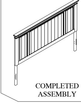
Step 1 :Attach and tighten the Leg Post (L/R) (B) to the Head Board (A).Insert JCBB (M8) With Washer (C&D) to affix.
