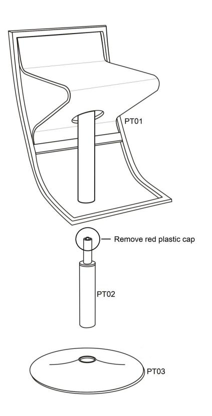
Lay the base (PT03) flat on the ground face up. Insert the pole (PT02) into the round hole in the center of the base (PT03) as shown in the drawing. Remove the red plastic cap at the top of the lift pole section (PT02). Carefully place the seat (PT01) on top of the lift pole (PT02) by inserting the lift pole (PT02) into the pole of the seat portion (PT01).
