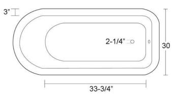
Dimensions of fixture are nominal and may vary within the range of tolerances established by ANSI Standard A112.19.2. Dimensions and specifications subject to change without notice.
