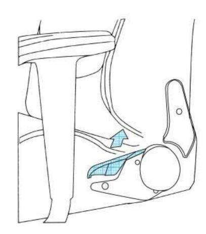
When tilting down the backrest to 180 degrees (if vigorously laying down), you may hear noises of clicking. It's from the gear rotating, not a defect of the product.
