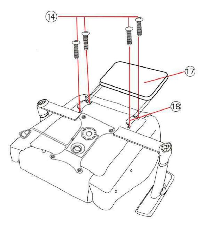
\* 14 Screws have been assembled on the seat, please loosen them for further assembly.\*
