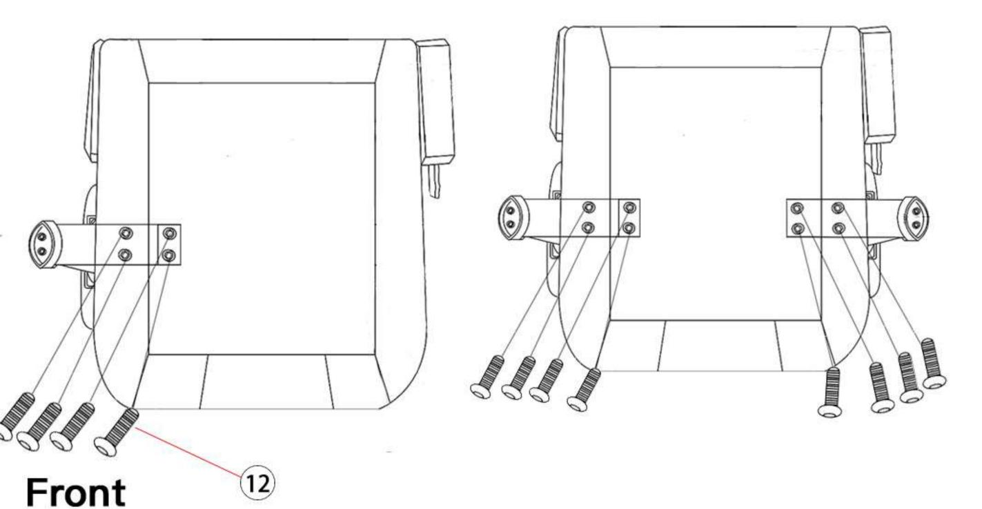
\* Screws have been assembled on the seat bottom, please loosen them for further assembly.\*
