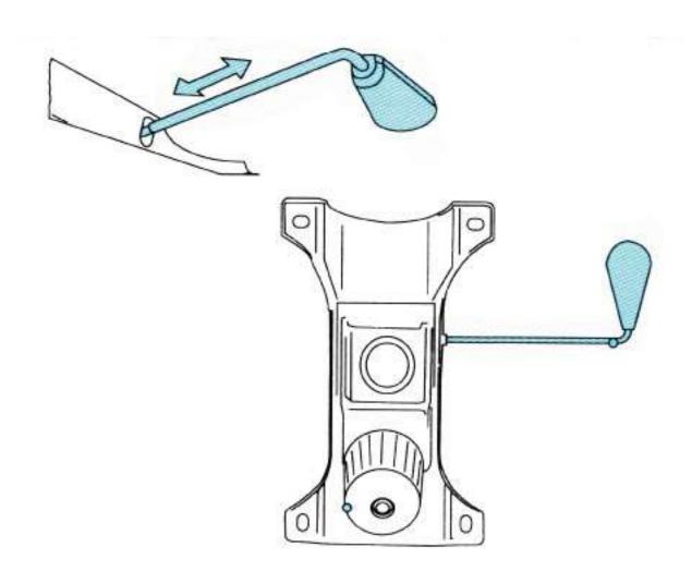
Put out/push in the lever to enable/disable rocking function
