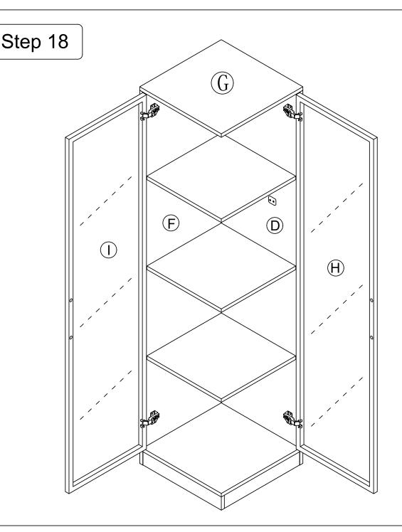
Turning this screw can effectively adjust the size of the door gap.
