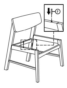
a) Insert Wood Dowel (F) into the designated hole on top rail of Side Frame.
