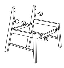
Attach Stretcher (3) to Right Side Frame (1) and Left Side Frame (2). Check that the screw hole on (3) is not facing up.
