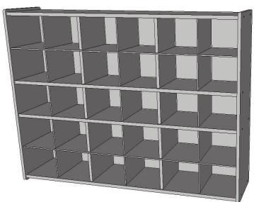
**Step 6:** Set unit upright, resting edges of Sides on floor. Tighten all screws snugly. **DO NOT OVER-TIGHTEN. DO NOT DRILL.** Assembly is now complete.
