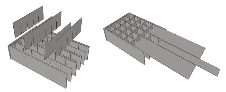
Step 3: Attach (2) 5/8" thick dividers to Top and Bottom pieces using (8) supplied Hex screws and Allen wrench. Slots in 5/8" thick dividers scissor into 5/8" wide slots in shelf pieces. Backs of dividers, (top of dividers pictured above), sit below back grooves in Top and Bottom pieces. Repeat for (3) 1/8" thick dividers. No hardware is required to attach 1/8" thick dividers.
