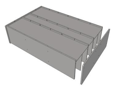
**Step 5:** Attach second **Side** piece using **(8)** supplied Hex screws and Allen wrench. Overhang on backs past Top, Bottom, and shelves will fit into deeper 3/8" back groove of second Side piece.
