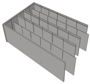
**Step 2:** Slide **(2) 1/8" thick shelves** into place between 5/8" thick shelves and Top and Bottom. No hardware is required in this step.
