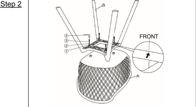
Place the Chair Seat (A) with its bottom side facing upwards onto a clean, soft surface to avoid any scratches or damage to the product.
