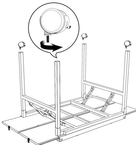
① Screw the wheels onto the legs.
