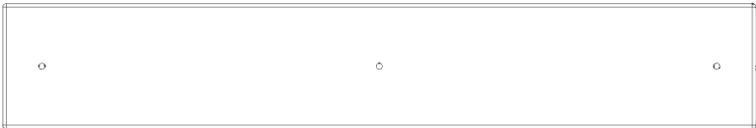
Y01 COVER BOARD - W4L19679 (x2) 5/8"x4"x24 3/16" (16x102x614)
