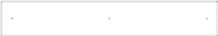
Y01 COVER BOARD - W4L19679 (x2) 5/8"x4"x24 3/16" (16x102x614)
