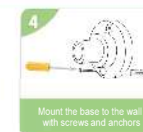
Mount the base to the wall with screws and anchors
