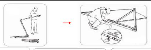
3. After making sure the legs are secure to the frame, using two people, lift the screen up in a vertical position. While the screen is in a vertical position, fold the front teet of the legs out
