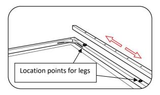
Step 2: Once you have aligned the leg's holes with the frame's holes, secure with the knob screws.
