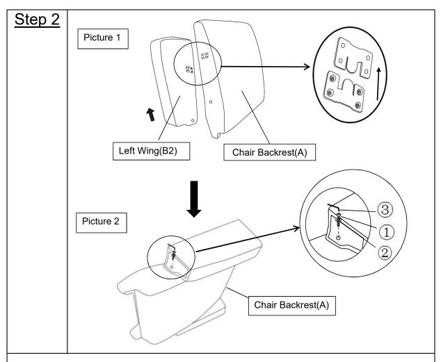
Align the mounting position of the Left Wing(B2) to the left side of Chair Backrest(A) .Then slide Left Wing(B2) forward by hand to make sure it locks into the position as shown in the picture 1.
