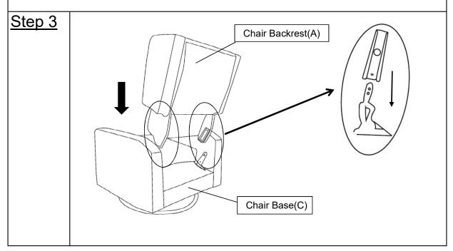
With assistance from your adult partner,hold up the fully assembled backrest with Wings,stand behind the chair.Insert the small Metal Arms on the sides of the Chair Backrest(A) into the prefabricated slide lock gadget on the Chair Base(C) as shown above.
