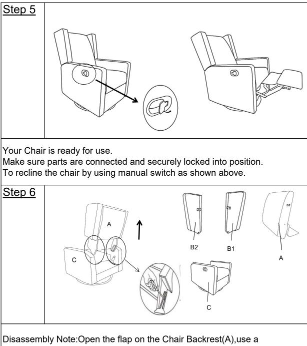
Disassembly Note:Open the flap on the Chair Backrest(A), use a screwdriver(Don't use fingers)pressing outward on the metal ear on the preattached Metal Bracket on one side of the Chair Base(C), with assistance of your adult partner to keep the Chair Base(C) in place, pull out the Chair Backrest(A) upward at the same time, repeat the same step for another side. Then the Chair Backrest(A) can be taken out.
