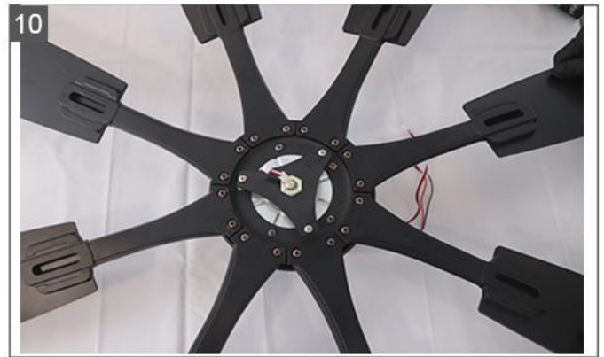
Repeat the previous step to complete the installation of all eight sets of fan blades
