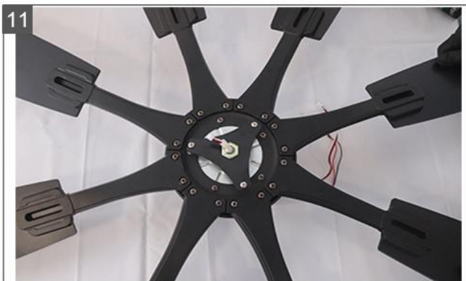
The connection between the fan blades and the motor is completed
