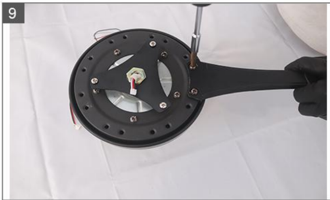
Securely tighten the fan blades (the side with the fork should face up). If the blade fork is installed in the wrong direction, there will be abnormal noise. And the motor, using the screws removed in step 6
