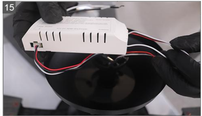
15 As shown in the figure, connect the two light source line interfaces and the motor line interface correspondingly
