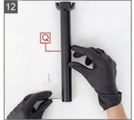
12 Put the pin back in the piece Q.
