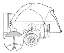
3. Secure the J hooks on the appropriate areas of the truck body.
