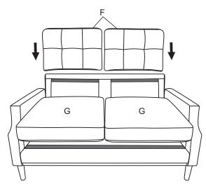
4. Tear out the Hook and loop fasteners on the frame, then stick with seat cushions (Part G ) & back cushions (Part F) and tidy them ok.
