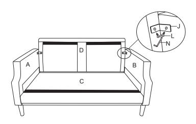
Connect the back frame (Part D) by aligning the metal piece (Part J) on Arms (Part A&B), then install Screw (Part L) with Toll (Part N)
