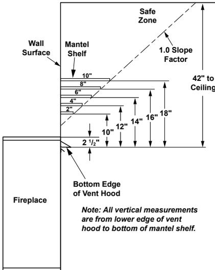
**Figure 3 - Minimum Mantel Clearances for Built-In Installation**
