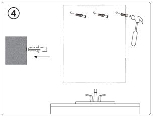
• Plug the plastic anchors into the holes.
