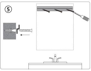
• Fasten the mounting bracket to the wall.
