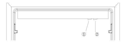
Light switch positions are like the above picture showed to control the backlight turn on/off:
