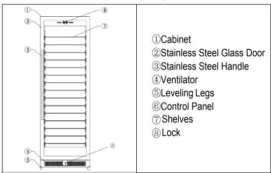
Note: EL-WCU107-02 is with right hinge, the handle is on the left. EL-WCU109-02 is with left hinge, the handle is on the right.
