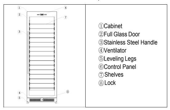
Note: EL-WCU106-02 is with right hinge, the handle is on the left. EL-WCU108-02 is with left hinge, the handle is on the right.
