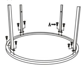
Step 2) Attach big open ring to long legs by using screw (B) and washer (C) as below shown. Tighten all screws firmly.
