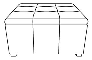
Place the Storage Ottoman right side up, test for eveness. Where you find this Storage Ottoman being uneven, identify the corresponding leg and "add or remove" a Washer Ring to achieve evenness.
