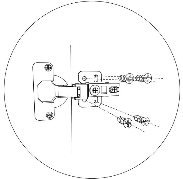
To prevent the door hinge from falling off, please install 4 screws
