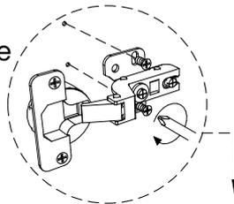
After completing the adjustments, please install the remaining two self-tapping screws
