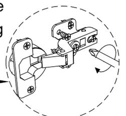
If there is misalignment after you install, adjust the screw to the best condition
