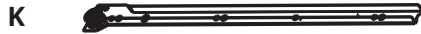
Outer Drawer Runner Left x 5 This runner attaches to the main body of chest
