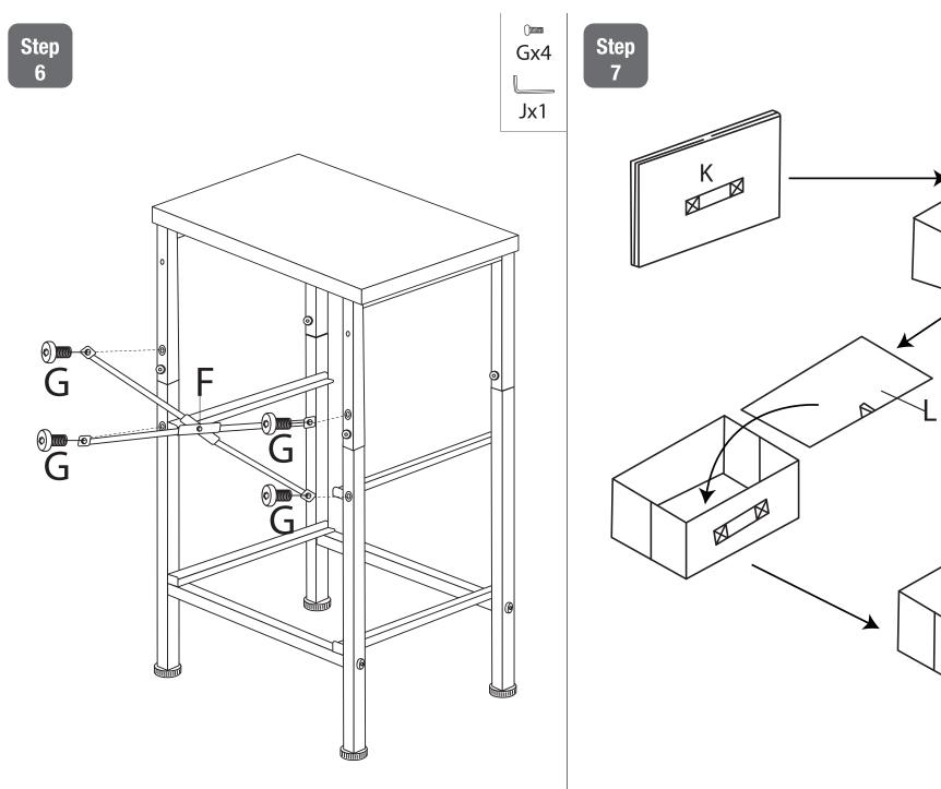
**Step 6:** Unfold rear bar (F) then place over assembled frame. Secure with short screws (G) using the hex key (J).
