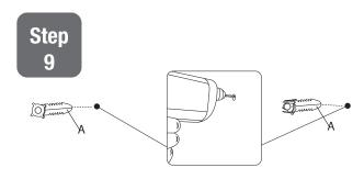
**Step 9:** Drill a hole into the wall using a 6mm bit and gently insert the wall anchor (A) with the help of a hammer.
