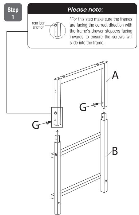
**Step 1:** Connect top frame (A)\* to bottom left frame (B) as shown. Secure with short screw (G) and tighten with hex key (J).
