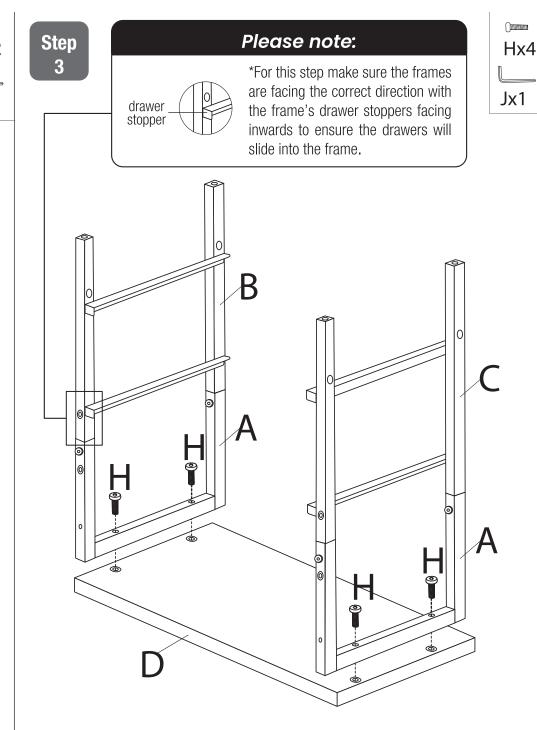
**Step 3:** Place assembled frames (A,B,C) over drawer top (D) as shown and secure with long screws (H) and hex key (J).
