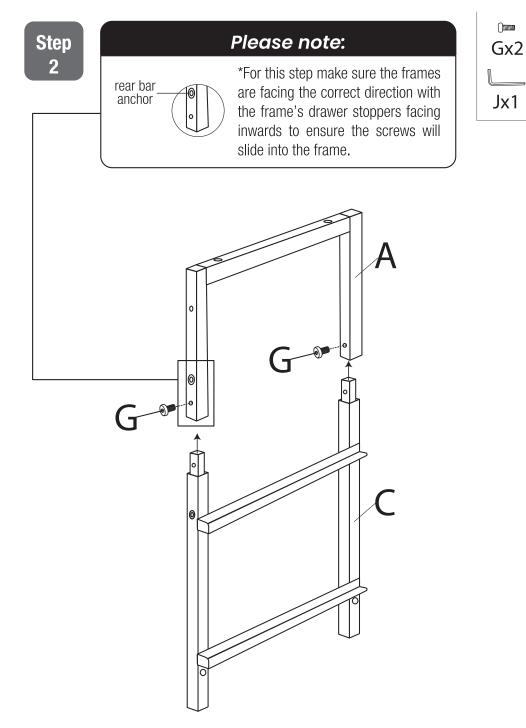
**Step 2:** Connect top frame (A)\* to bottom right frame (C) as shown. Secure with short screw (G) and tighten with hex key (J).
