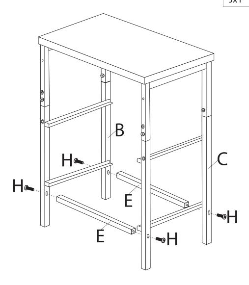
**Step 4:** Connect frame poles (E) to frames (B,C) and secure with long screws (H) and hex key (J).
