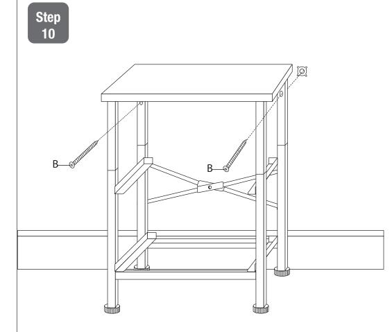
**Step 10:** Place the shelf against the wall, and insert the wall mount screws (B). After making sure everything is screwed in tightly, you can start to use the assembled piece. Enjoy!
