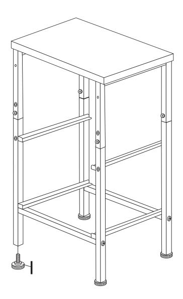
**Step 5:** Screw frame screws (I) into the legs of the assembled frame.
