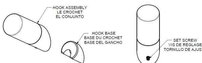
Place hook assembly over base. Attach hook to base with set screw.
