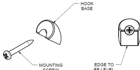
Place hook base in desired location. Position bottom edge to be level. Mark mounting hole location. Drill 3/32" pilot hole. Fasten hook base to wall using screw provided.
