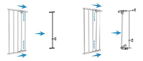
**4-2** The first and last inserts of the door frame are connected
