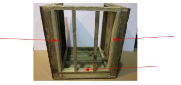
3. Now you should have the bottom part of your storage unit built, to build the top section you will now need the remaining **back board** (larger) and the **angled sideboards**. Screw together as per diagram.
