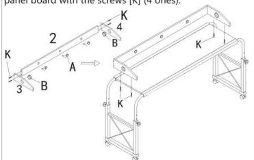
Step 4: Fix the parts finished in the above step onto the back of the panel board with the screws [J]
