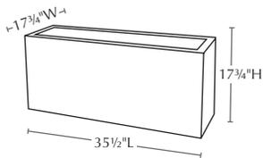
**Materials:** unsaturated polyester resin, sand, stone powder, talc powder, and fiberglass
