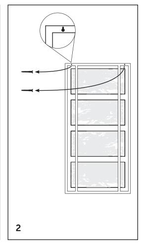
Measure the distance between the two holes on the back of Mixed Wood Wall Panel.
