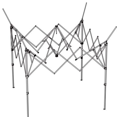
**EN** Open the canopy frame. With two persons on the diagonal ends, lift and partially pull the canopy frame apart.
