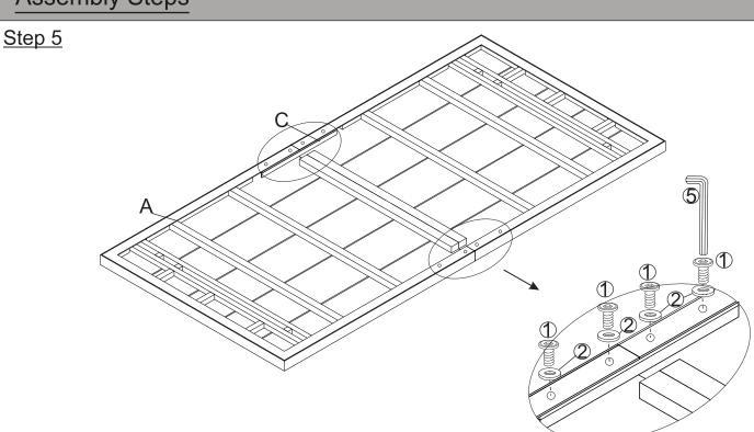
Secure the Support Bar (C) to the Table Top (A) by using the Bolts (1), Washer (2) and Allen Key (5) as shown in the picture.
