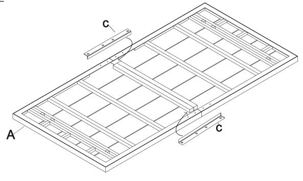
Place Support Bar (C) underside of long apron of Table Top (A) as show in picture above.
