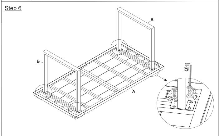
Attach the Legs Frame (B) to the Table Top (A) using the Bolts (1) with Washers (2) and Allen Key (5) as shown in the picture.
