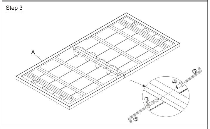
Secure Table Top (A) using the Bolt (3), Sleeve Nut (4) and Allen Key (5) as shown in the picture.
